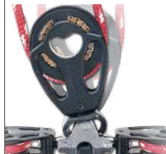
Control blocks attach to ears to reduce load on car.
