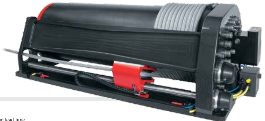
Two inner magnetic switches factory-set at the feeder's stroke limits prevent overtravel. Two outer fail-safe limit switches automatically engage the brake.
