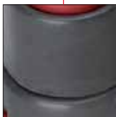
6061-T6 aluminum: Hard Lube-anodized
