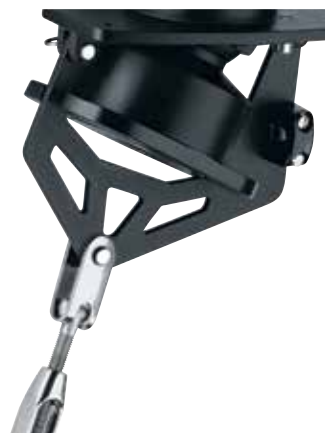
Turnbuckle eye on stationary bracket attaches to an underdeck chainplate.
