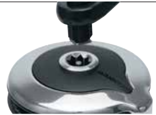
A Harken locking handle inserted into an unloaded winch automatically disconnects the motor gear for manual operation.
